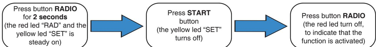
⚠ The activation of the self-test, without having properly connected the photocells to the control unit, will cause a malfunctioning of the system.
